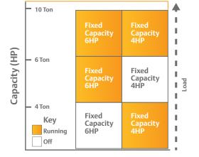
Uneven tandems can deliver three capacity stages to match the loads as the demand increases
