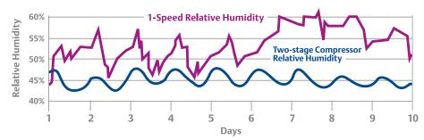
Field testing shows improved temperature and humidity control provided by Copeland Scroll two-stage compressors compared to fixed compressors.
