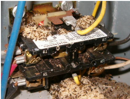
Open design allows for damage from fire ants, other insects.
