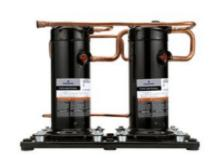
Multiple Copeland Scroll™ compressors are connected with a manifold in tandem or trio. This configuration is ideal for air conditioning applications wanting to achieve excellent part-load efficiency without the need for complex controls integration.
