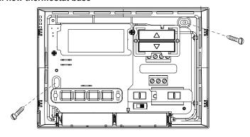
Mount your new thermostat base using the supplied screws. Drill holes and insert wall anchors to secure the thermostat base to the wall, if necessary.
