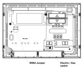
If you have either a gas or oil furnace, set the switch to GAS. If you have an electric furnace, set the switch to ELEC.
