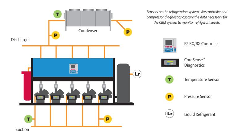
located in closed areas, remote leak detection monitors the complete refrigeration system by analyzing key refrigeration operating indicators to provide actionable intelligence.
