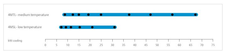
Conditions for 4MTL: EN12900 R744: Evaporating -10°C, Gas cooler exit: 35°C/ 90 bar, Superheat: 10K for medium temperature Conditions for 4MSL: EN12900 R744: Evaporating -35°C, Condensing -5°C, Superheat 10K, Subcooling 0K for low temperature
