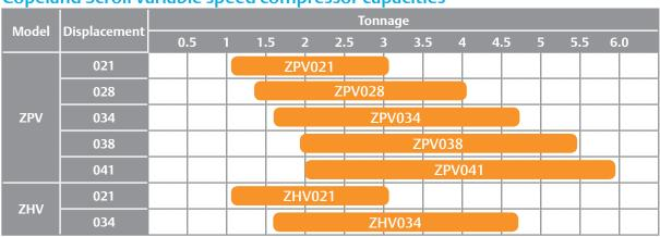
ZHV models for hot water heating applications. Capacities are at 50/115 operating conditions.
