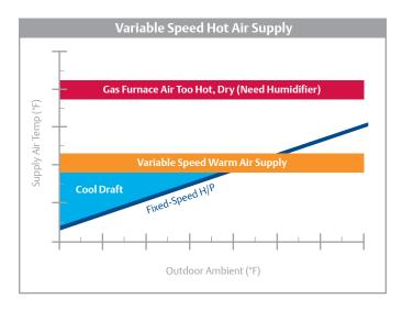
This unique compressor design enables heat pumps to supply hot air even during cold winter conditions
