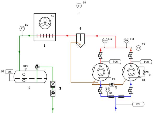
Figure 6: P&I diagram for OMTE-76D & OMTE-90D models
