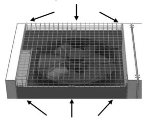
Figure 37: Opening the fan safety grid
