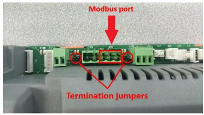
Figure 15: Modbus port and termination jumpers
