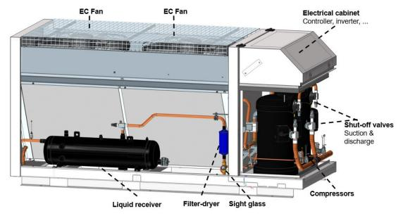
Figure 10: Main components of LOCU units
