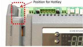
Figure 25: Location of "Hot Key" plug connection
