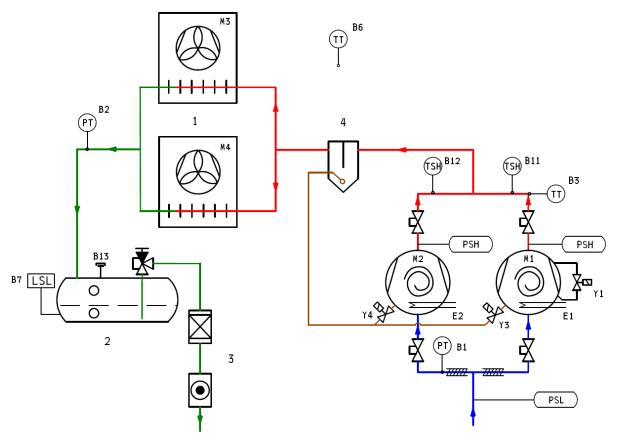
Figure 7: P&I diagram for OMTE-152D models
