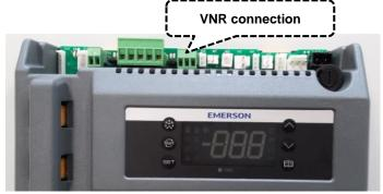
Figure 18: VNR connection for the remote display
