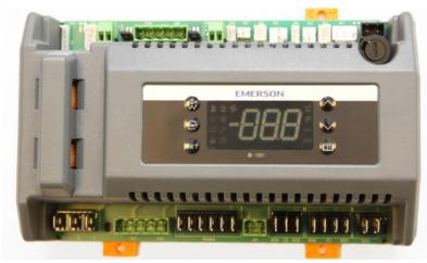
Figure 13: XCM25D Electronic controller
