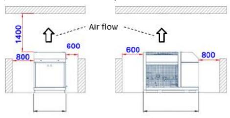
Figure 32: Fixing dimensions and distances in mm
