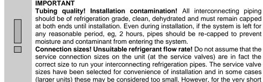
The piping should be sized to ensure optimum performance and good oil return. The sizing must also consider the full capacity range through which this unit will need to operate.
