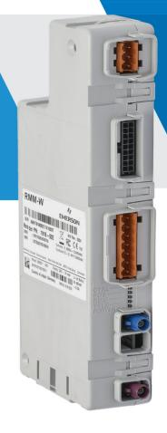
Emerson's RMM-W modems are fitted with a Global Navigation Satellite System (GNSS) for the best around the world coverage. Accurate positioning and tracking information ensures visibility of your assets, valuable information in the event of claims, managing ETA's and monitoring current locations.
