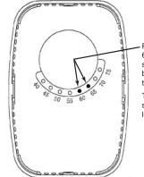
Pins are shown installed at 60 and 65°. The temperature setting range is limited between these two temperatures.
