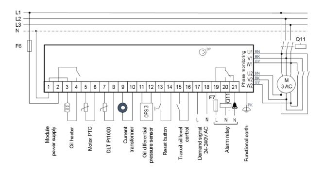
\*1-2 Power Supply, 19-20 Control circuit & 17-18 Welded contact alarm (optional)
