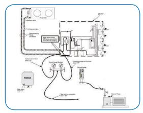
Remember that the refrigerant is under pressure. Always wear protective equipment, i.e. safety glasses or goggles and gloves when working with refrigerant, and guard against refrigerant spraying into the face or skin. Line pressures on an operating conditioning unit will vary with outdoor temperatures. As outdoor temperatures rise, pressures will also rise.
