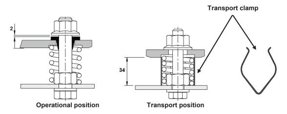
Due to differences in weight (cylinder / motor side) different springs have been used on both sides. Springs have different colours for easier identification: violet on motor side and orange on cylinder side.
