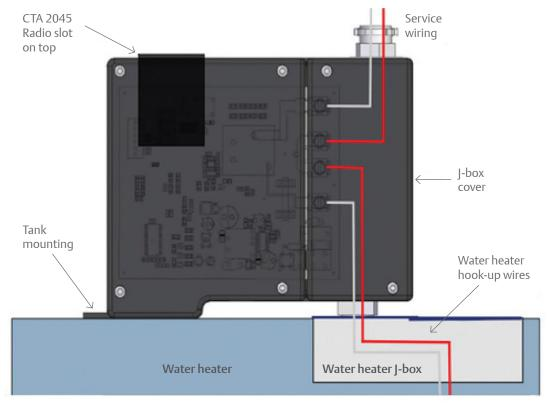
Patented design mounts directly to water heater
