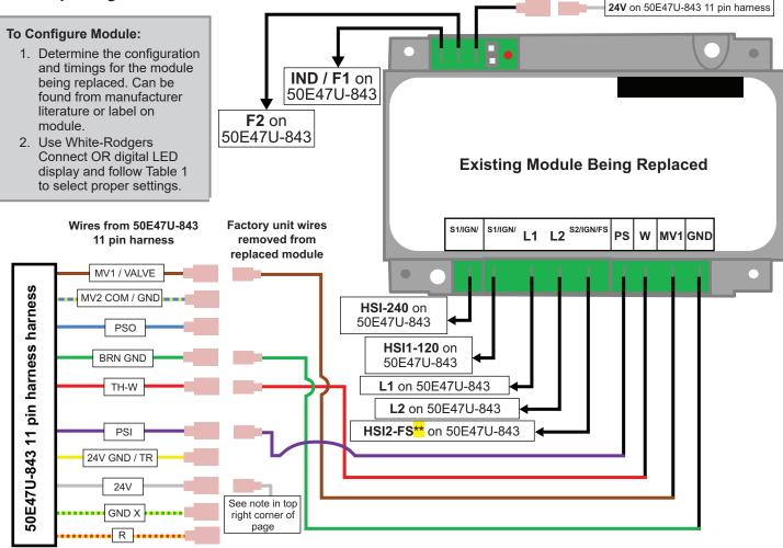
For remote sense applications, connect the neutral side of the ignitor to the transformer 120V neutral (off board) and connect the remote flame sensor from S2/FS to SENSE on 50E47U-843
