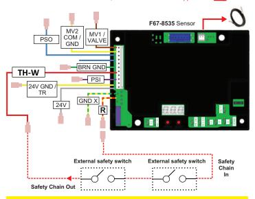
IMPORTANT: Connect R on 50E47U-843 module to input of safety switches (limit, rollout, etc.) and connect output of safety switches to TH-W on 50E47U-843
