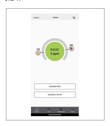
Check the CRLDS mobile app home tab to verify the PPM reading and alarm state while gas is flowing.
