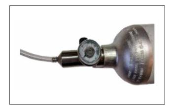
Use the gas regulator with constant flow of 0.5 L/min.
