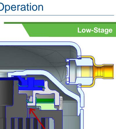
Vent Holes Open Bypassing Outer Portion Of Scroll
