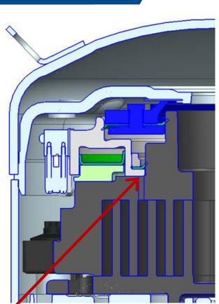
Vent Holes Closed Utilizing Full Scroll For Compression
